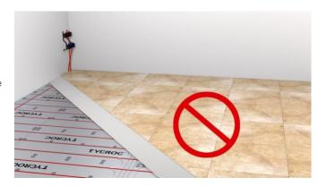
The use of ceramic tiles and natural stone is **ALLOWED ONLY** if the Tycroc UHP panels have been installed using the gluing method.
