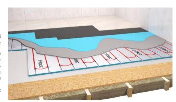
It is **STRICTLY PROHIBITED** to use ceramic tiles or natural stone if the Tycroc UHP panels have been installed using the screwing method.
