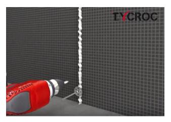
For fastening of building board use Tycroc screws M4x35mm or M4x55 mm and Tycroc metal washers 36x0,6 mm should be used. Use screws that enter the underlying surface by at least 20 mm.
