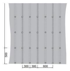
A) / B) Place building board on the floor and press it strongly against the surface, fixing the building board with suitable screws and metal washers 36x0,6 mm. Use screws that enter the underlying surface by at least 20 mm.
