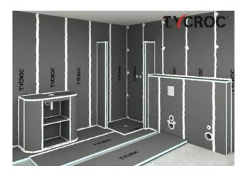
4.3 Place the Tycroc TWP building board on the floor and press it strongly against the surface either by body weight or using additional weight (e.g. a bag of concrete, etc.). Before mounting the next board, Tycroc Premium FIX adhesive sealant should be applied to the edge of the previous board to glue the building boards to each other.
